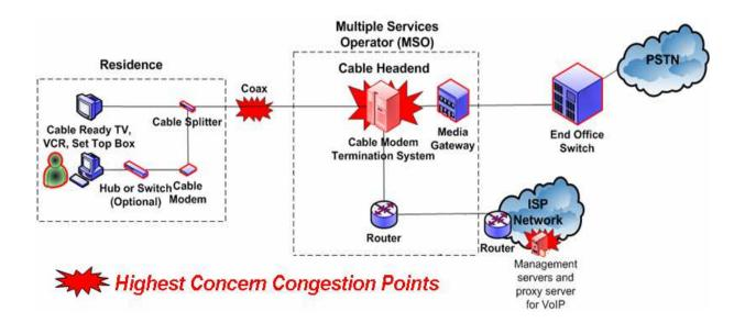
Figure 4.3-2 Potential Congestion Points for Typical Cable Modem Architecture [12]
