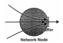
Figure 4.1-2 Traffic Aggregation Congestion in a Network Node [11]
