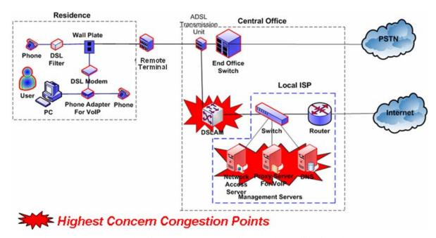
Figure 4.3-1 Potential Congestion Points for Typical DSL Architecture [12]
